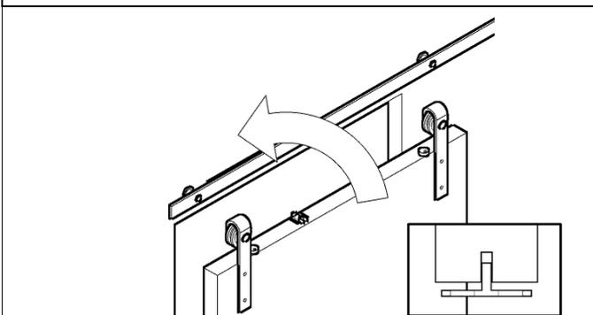
**STEP 9:** Adjust the trigger into the final position and tighten the screws.
