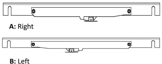
**STEP 5:** Loosen end two fixings. Slot Soft Close onto standoffs.
