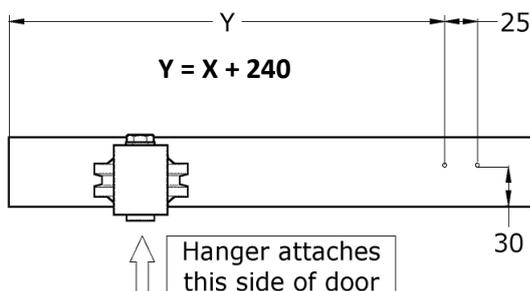
**STEP 4:** Install the Soft Close in correct orientation.
