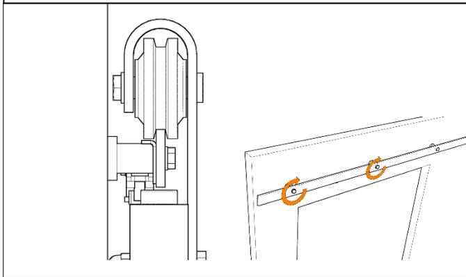
**STEP 7:** Loosely install the trigger on top of the door pushing it as far forward as possible.
