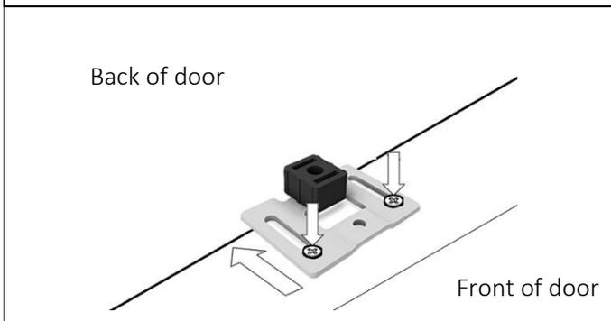
**STEP 8:** Hang the door back on the track, ensuring the floor guide is engaged.
